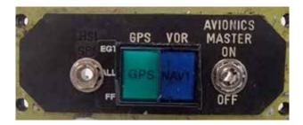
Figure 4 HSI Source Annunciator Lights
