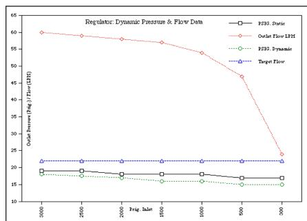
Our regulators have a virtually flat outlet pressure regulation curve for both lock-up (static) and flowing (dynamic) with inlet pressures from 300 to 3,000 psig. In open and closed-loop instantaneous flow tests, they have very well dampened, oscillation free flows. Flows of 55 to 60 liters/minute are measured through a controlled pneumatic resistance with inlet pressures of 1,000 to 3,000 psig. Target flows are 22  $\pm 2$  liters/minute throughout the inlet pressure range of 500 to 3,000 psig.
