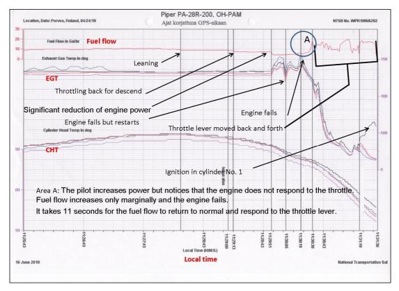
Figure 11. Engine parameter analysis from the terminal phase of the flight.
