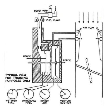
Figure 9. A schematic diagram of a Bendix RSA-5AD1 fuel injector unit. The picture does not show the idle valve (power control), the mixture valve or the connecting rod from the throttle valve to the idle valve. Picture: Precision Airmotive Corporation.
