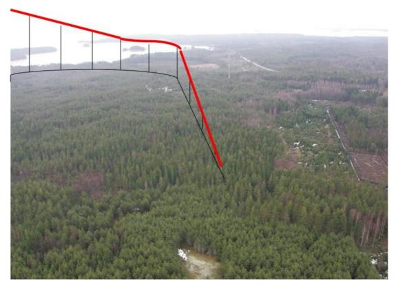
Figure 6. Aerial photo of the accident area. The red line indicates the trajectory in the air and the black line shows the flight path superimposed onto the terrain. The GSM mast is also visible in the photo.
