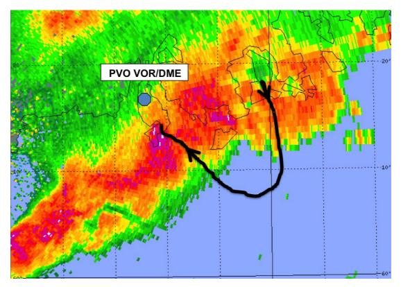
Figure 7. The aircraft's track and the rain / snow area at 11:30.
