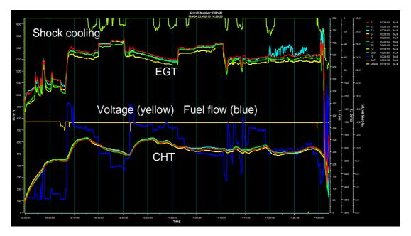
Figure 5. EDM-recorded engine parameters for the entire flight. The parameters can be studied in detail by zooming into them with the manufacturer's analysis program. A more detailed analysis of the parameters is presented in figure 11.
