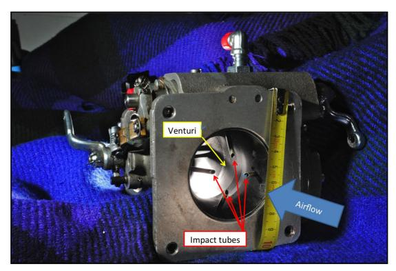
Figure 10. A Bendix RSA-5AD1 fuel injector unit.
