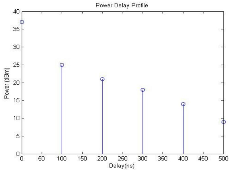
**Figure 2.8 Discrete Power delay profile**
