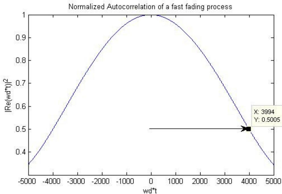
**Figure 3.4 Autocorrelation of the channel (Rural Environment)**
