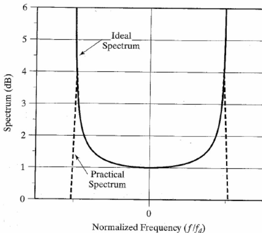
Figure 2.5 Ideal (Equation 2.16) vs. Practical Doppler spectrum
