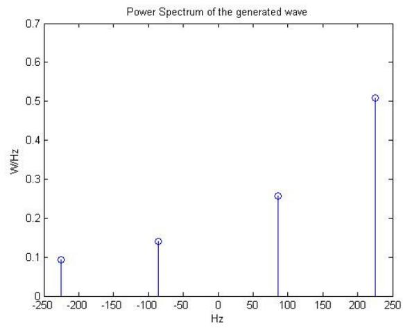
**Figure 5.8 Spectrum of the channel ( $v=150$  km/h)**
