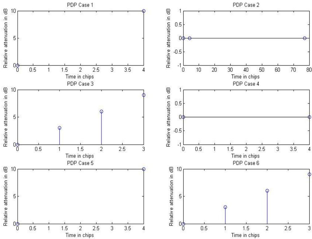
**Figure 4.1 PDP of each case**
