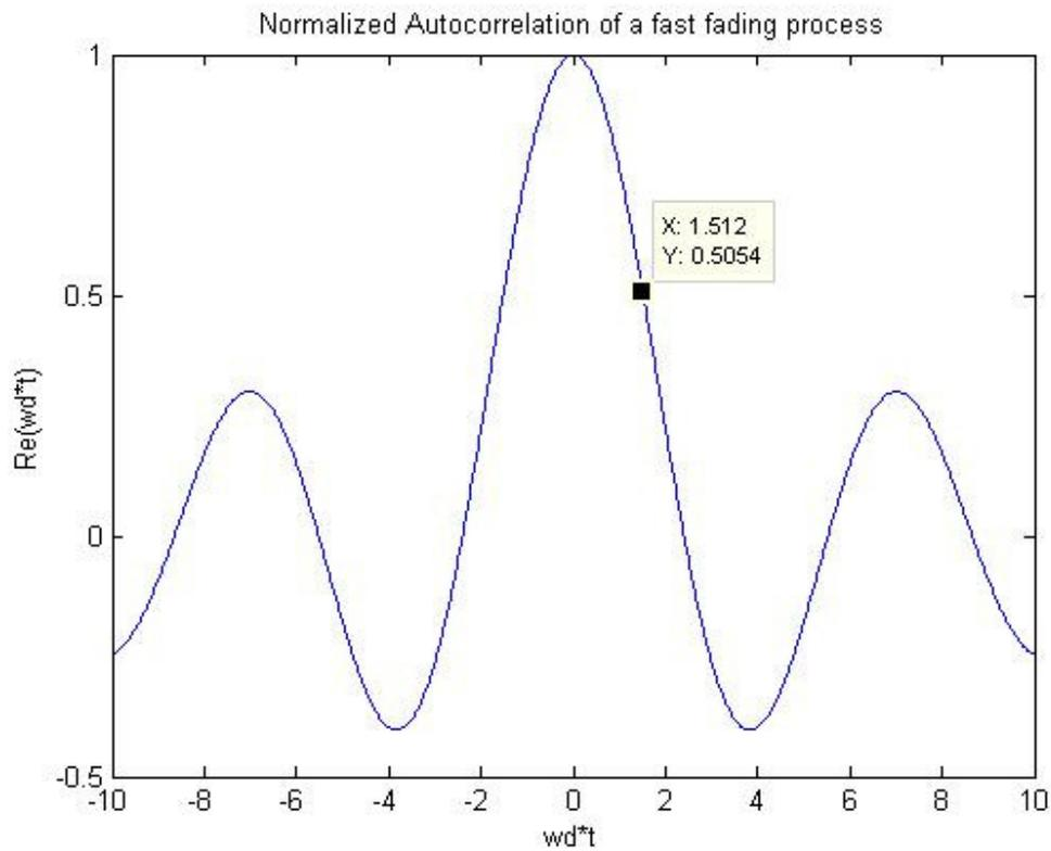
Figure 3.2 Autocorrelation function of the channel (Clarke's Model)
