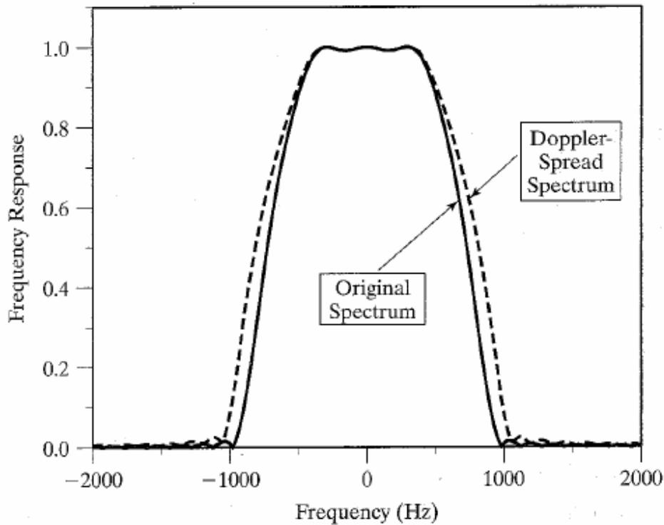
Figure 2.7 Doppler Spread Spectrum
