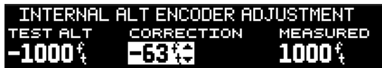
Figure 7-15 Internal Alt Encoder Adjustment
