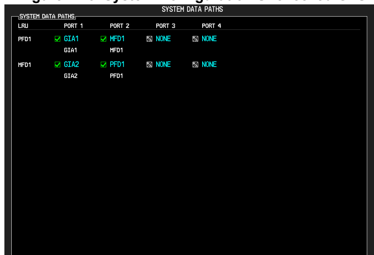
Figure 7-44 HSDB System Data Paths Unchecked GTS
