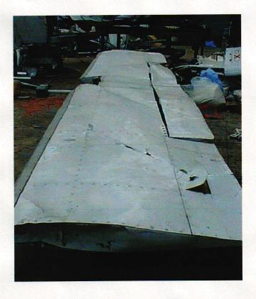
Picture 6: Horizontal stabilizer. Note the deformation towards the rear, the buckled trim tabs and the scar on the left hand side.
