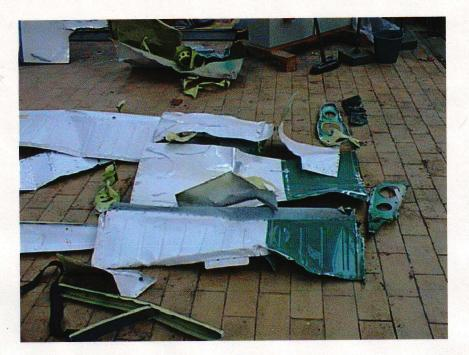
Picture 5: Remains of the upper wing skin and aileron of the right hand wing tip.
