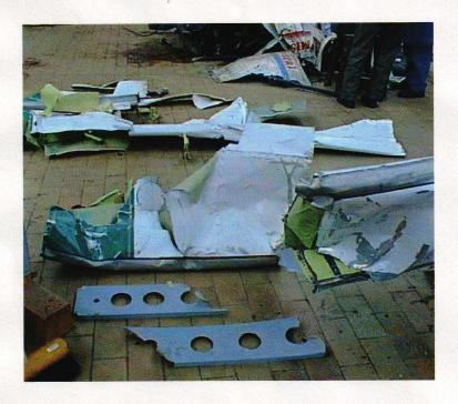
Picture 4: Leading edge of the right hand wing tip. The nose of the leading edge shows clearly that the wing skin has been "rolled up" towards the top.
