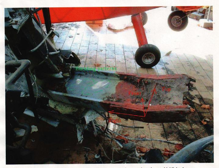
Right hand portion of main spar. Buckling patterns and parts orientation are highlighted. The bent hydraulic tubes and control rods are clearly visible. Picture 2:
