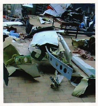
Picture 3: Remains of the left hand wing. The main spar is bent towards the top and the rear.
