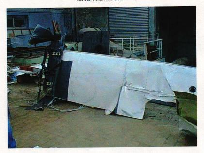
Picture 1: Top view of the right hand wing. Note the bent fuselage sides at the wing root.
